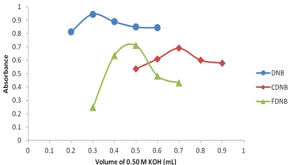
Figure 5: Effect of volume of 0.50 M ethanolic KOH on the absorbance intensity of the reaction products of 10  $\mu\text{g/mL}$  NAB with 10 mg/mL DNB, 160  $\mu\text{g/mL}$  NAB with 10 mg/mL CDNB and 30  $\mu\text{g/mL}$  NAB with 1% v/v FDNB.
