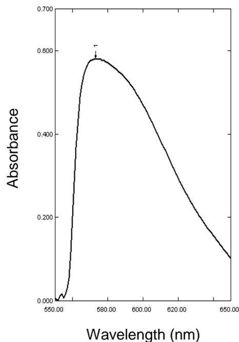
**Figure 3: Absorption spectrum of the reaction product of 30 µg/mL NAB with FDNB in DMSO.**
