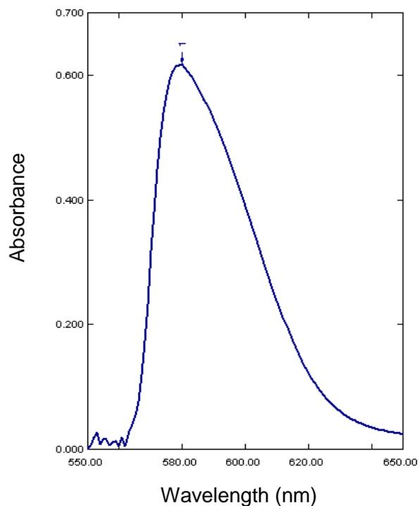
Figure 1: Absorption spectrum of the reaction product of 6 µg/mL NAB with DNB in DMF.
