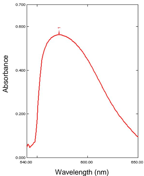
Figure 2: Absorption spectrum of the reaction product of 120 µg/mL NAB with CDNB in DMSO.
