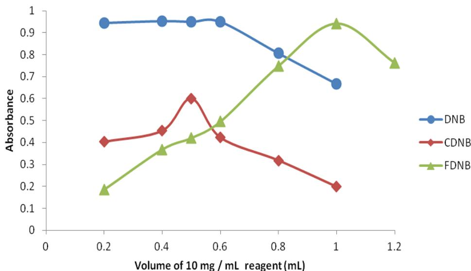
**Figure 4: Effect of volume of reagents on the absorbance intensity of the reaction products of 10  $\mu\text{g/mL}$  NAB with 10 mg/mL DNB, 120  $\mu\text{g/mL}$  NAB with 10 mg/mL CDNB and 50  $\mu\text{g/mL}$  NAB with 1% v/v FDNB.**
